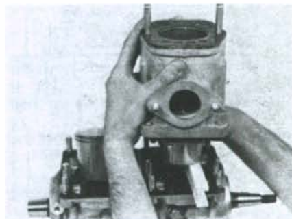
Fig. 30—Use a suitable ring compressor to install cylinders.
