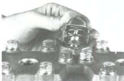
Fig. 34—Installing thermostat in liquid cooled engine.
