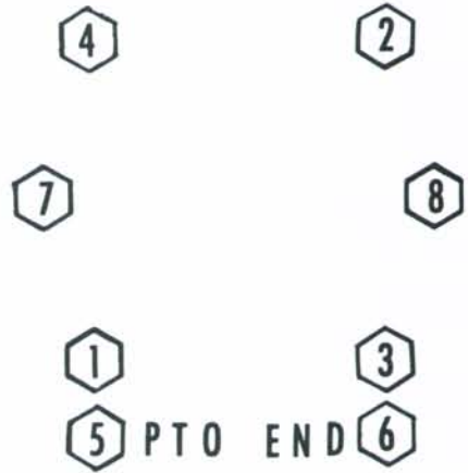
Fig. 11—Tighten crankcase retaining cap screws in the sequence shown. Refer to text for tightening torques of the various sized screws.
