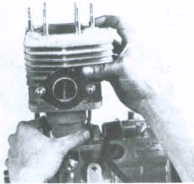
Fig. 7—Lifting off the cylinder block on single cylinder engine.
