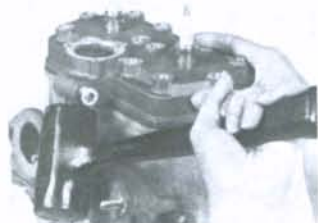
Fig. 26—Removing cylinder head on liquid-cooled engine.
